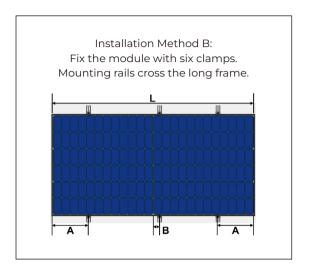
The Maximum Test Load of Mono-Facial Module Installation
